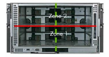
The enclosure comes preinstalled with removable full-height dividers between the top four device bays and the bottom four device bays. In addition, there is a half-height divider available for use between device bays 4 and 8 if the full-height divider is removed. Using these combinations of dividers, the following combinations of server blades can be installed:
